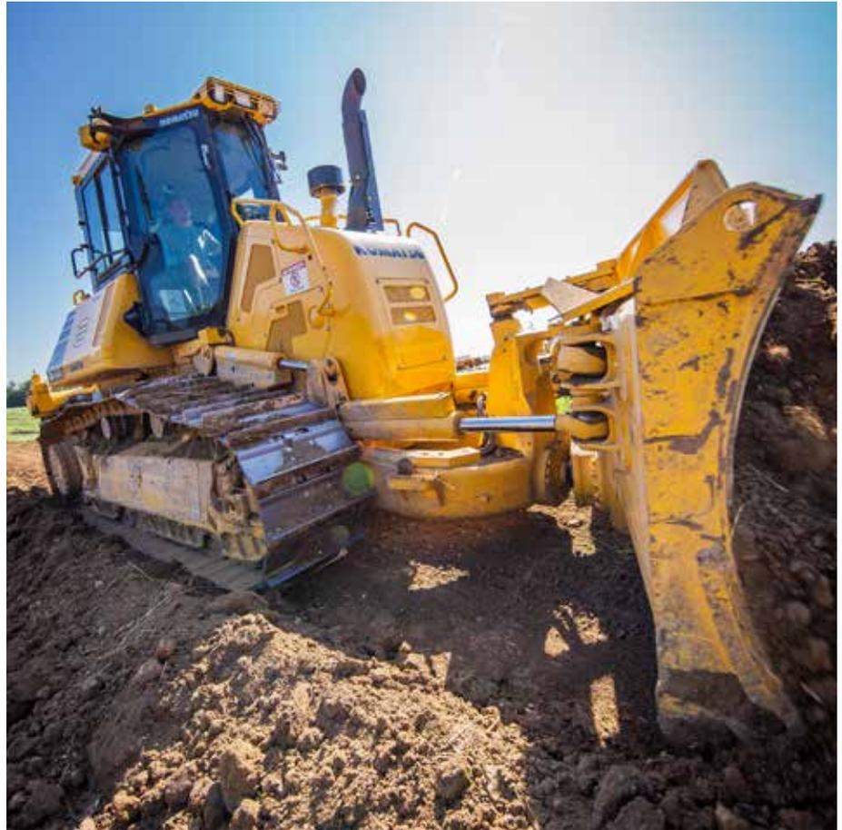
A Pullins Drainage Komatsu D61EXi makes short and accurate work of farmland re-grading in South Vienna, OH. The project involved over 2,500 feet of 40- and 30-foot wide erosion-control waterways. With Komatsu iMC, Operator Kole Wilbur enjoys completing the task in fewer passes.
